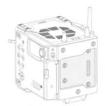
The battery adapters attach to the recessed area at the rear of the camera with four captive M4 screws.
