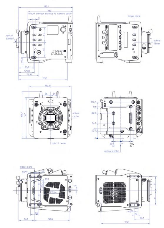
Camera body with LPL lens mount. All dimensions in mm. Not to scale.
