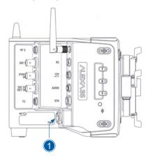
The PWR 8pin LEMO connector (1) is at the right side of the camera. Use KC50-S (K2.75007.0) or KC50-SP-S (K2.0001275) power cables to connect the camera to a power supply.
