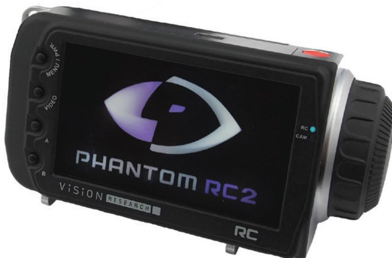
The Phantom Remote Control Unit (RCU) is a small, lightweight, hand-held controller which allows you to adjust most settings on your camera as well as view and save recorded cines to the CineMag IV. The RCU is available in both wired and wireless versions. Both versions will connect with an included 5 meter cable direct to the back of the camera. Alternatively, the wireless model includes a Bluetooth dongle that allows for operation from up to 100 meters.
