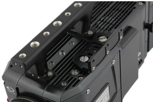
The adjustable arm mounts to the viewfinder, and then can be adjusted to the desired position on the camera body. An HD-SDI cable and 12V power cable are also included and connects to the front left side of the camera.
