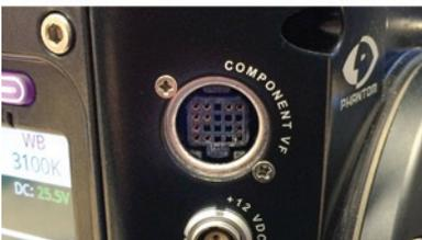
The component viewfinder port on the right side of the camera supplies 12V power and YPRPB component video. The standard connector is a Fischer 7-pin, which works with Sony HDVF30, HDVF35W (with a custom cable from Vision Research) and the Vision Research YPRPB monitor cable.
