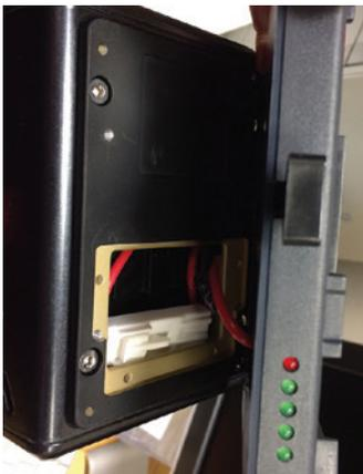
Once connected, attach the mount assembly to the 4 screws around the perimeter of the rear of the camera. (Note: the Anton Bauer mount does not have a second back panel assembly)
