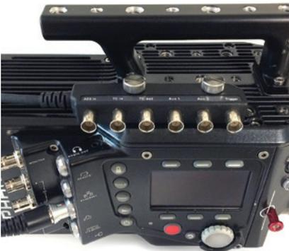
The Flex4K's Sync port is compatible with a multi-bnc capture cable and Phantom Mini-Break out Box (commonly known as the Mini-BOB). Both of these accessories provide the same functions, however the Mini-BOB is designed to mount to the top of the camera (as pictured) for better cable management.
