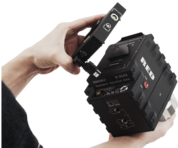
Figure: Install +1 Adaptor Module
