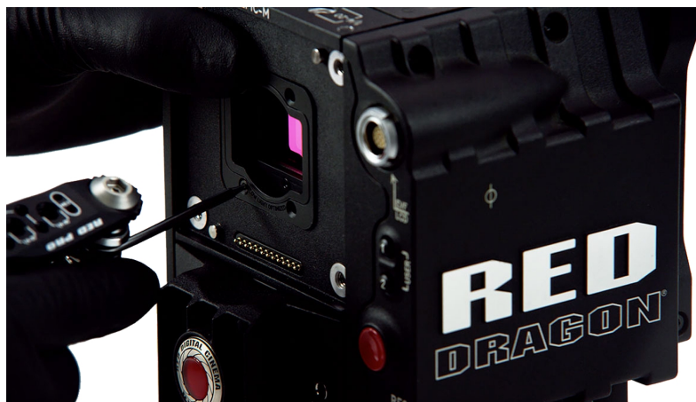
Figure: Replace the OLPF Module and Screws
