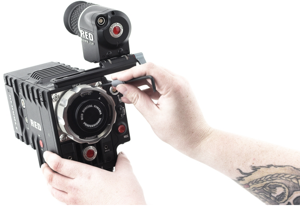
Figure: Remove the Lens Mount Screws
