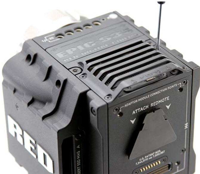
Figure: Replace the Hood Scoop
