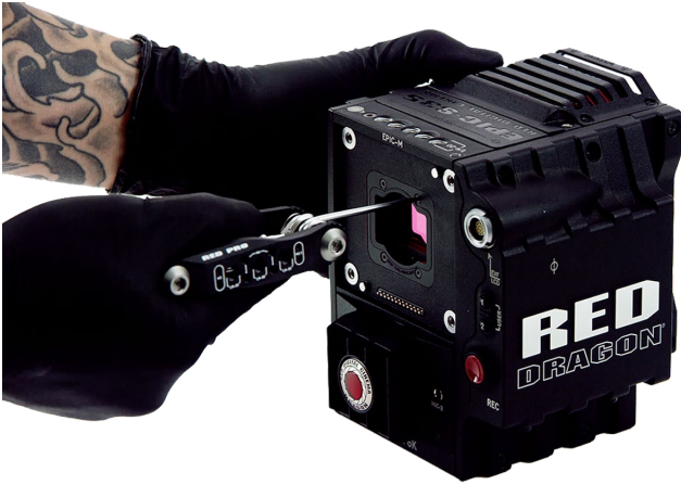
Figure: Remove OLPF Module Screws
