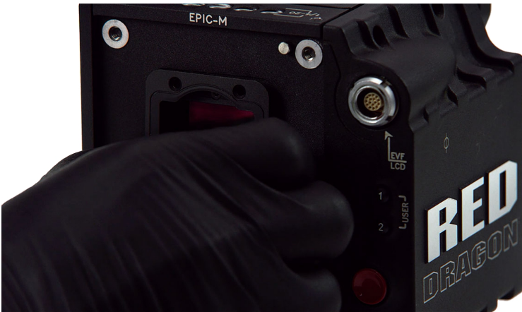
Figure: Remove the OLPF Module
