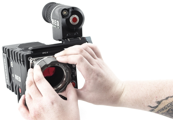
Figure: Remove the Lens Mount
