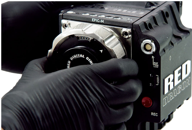
Figure: Remove Lens Mount
