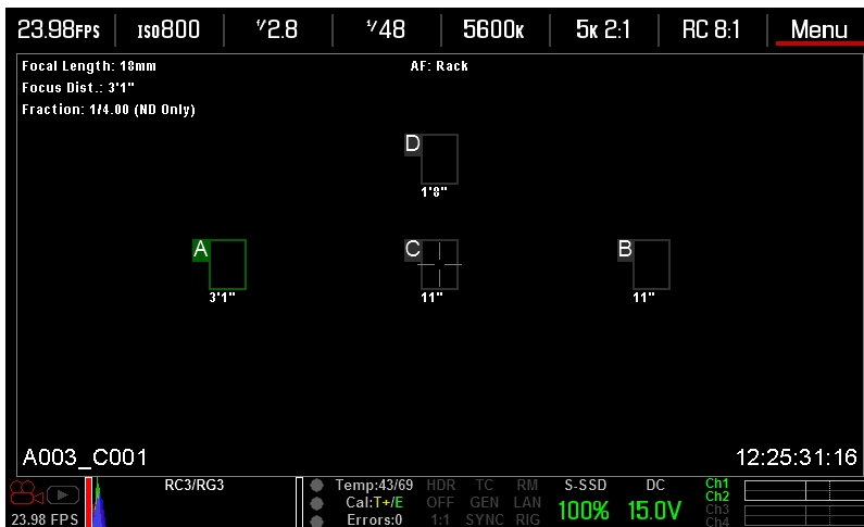
Figure: Set Rack Point Location
